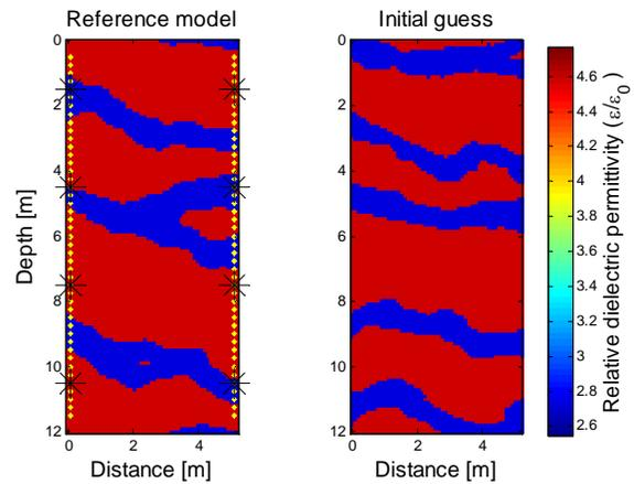
Figure 2. Left) Synthetic reference model. Black asterisks show transmitter positions and the yellow dots show receiver positions. Right) The initial model used as input for the inversion.
